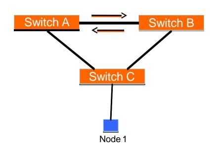
Switches A and B broadcast node 1's frame out every port
