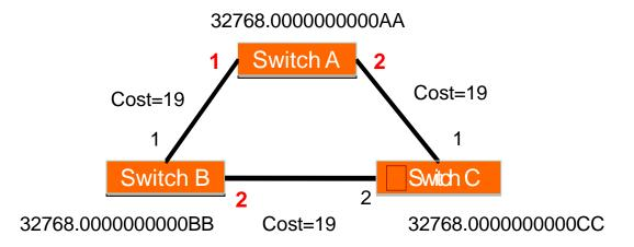
Port 2 in Switch C is then put into the *Blocking State* because it is *neither a Root Port nor a Designated Port*
