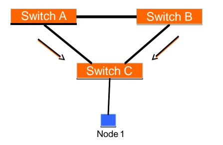
Switches A and B broadcast node 1's frame out every port
