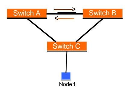
Switches A and B broadcast node 1's frame out every port
