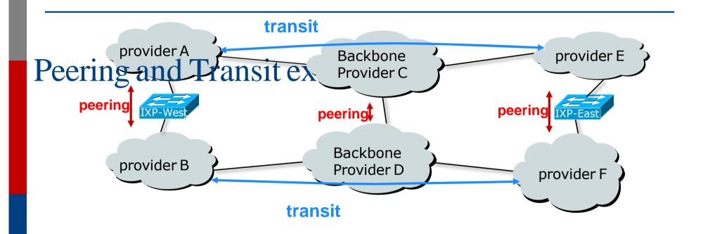
A and B peer for free, but need transit arrangements with C and D to get packets to/from E and F
